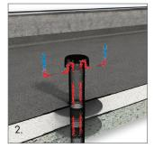
1. Installation example: Flavent® Single-piece breather vent for ventilated roof with PVC roof membrane
